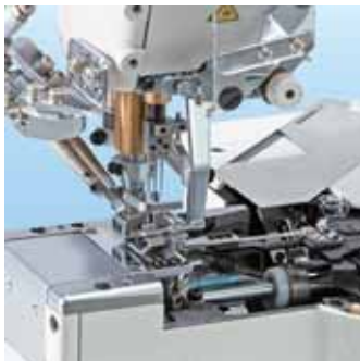
Pneumatic type top and bottom thread trimming mechanism
