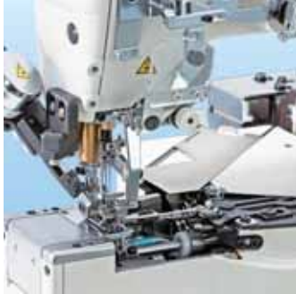
Electromagnetic type top and bottom thread trimming mechanism
